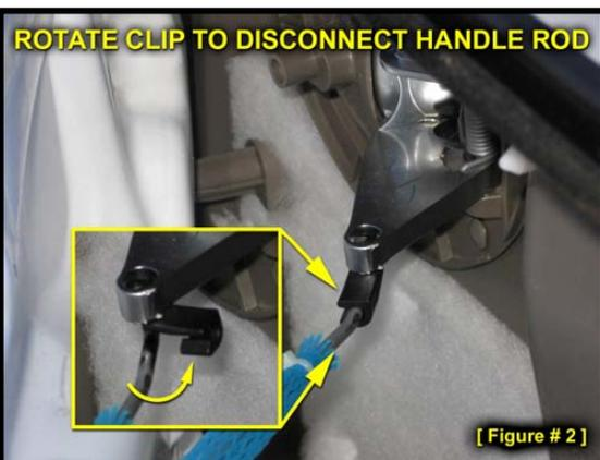
You should now be able to pull the panel far enough away from the door to reach behind it and disconnect the inside door handle actuating rod. To do so, simply unclip and rotate the plastic lock which will allow the metal rod to slip down and out of the hole. (Figure 2) Lift the panel up off the door lock knob and then set it aside.
